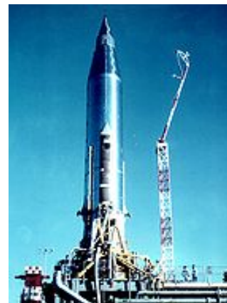
Atlas-B rocket with SCORE on the launch pad – The whole rocket body (without the booster engines) constituted the satellite SCORE.
