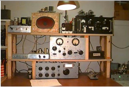
The rig shown above is N2EY's current homebrew setup, known as the Southgate Type 7. It's a 100-watt all-hollow-state CW transceiver for 80, 40 and 20 meters, and was built in the mid-1990s from 99% reused/recycled parts.
