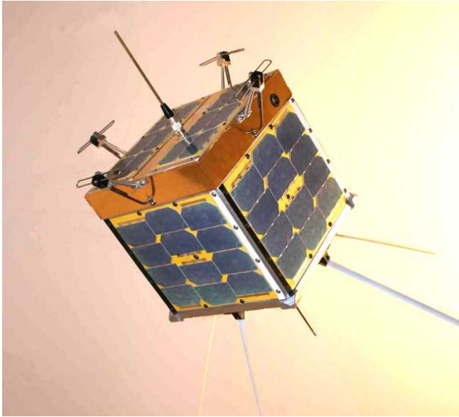
Amsat-ZL's KiwiSAT Amateur Radio satellite project. Mark 2 design with improved Solar cells and enlarged structure.
